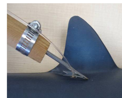
Fig 6: Dart tag with needle on tagging mount and downward-facing tag points. (Source: Cooperative Shark Tagging Program NOAA NFMS (NOAA 2017))
