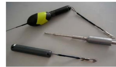
Fig 11: Pop-off satellite tags with dart tags and needle attachment for pole. (Source: Juerg Brunnschweiler)
