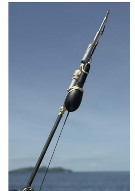
Fig 13: Pop-off satellite tags including dart tag mounted on a tagging pole. (Source: Juerg Brunnschweiler)
