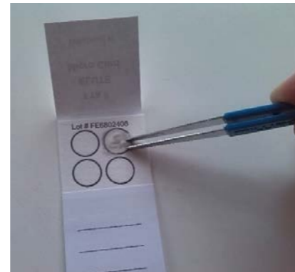
Fig 6: Squash a small piece of tissue onto the card. (Source: Sharon Appleyard, CSIRO)
