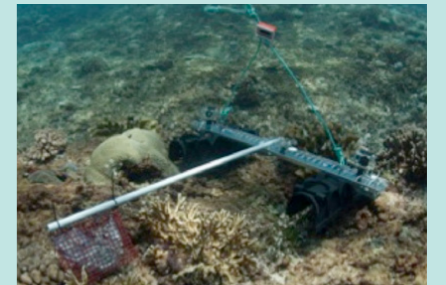
Fig 4: Acrylic BRUVS with a camera inside each plastic drain pipe. (Source: Vanessa Jaiteh)
