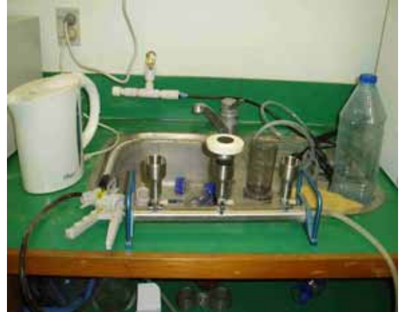
The spectrophotometer provided by Institute Pasture is used by TWB lab – that lacks the manual & consumables, not a very clean space to work. Also seen is the membrane filtration system for bacteriological analysis.
