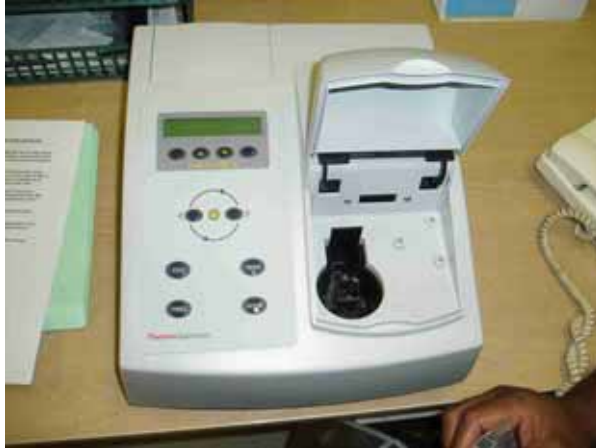
The spectrophotometer provided by Institute Pasture is used by TWB lab – that lacks the manual & consumables, not a very clean space to work. Also seen is the membrane filtration system for bacteriological analysis.
