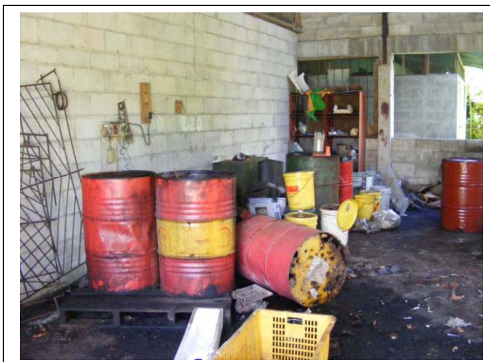
Figure 5 – visible oil stains from corroding drums
