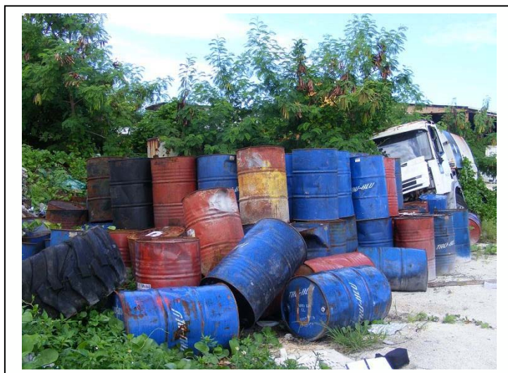
Figure 2 – multiple drums stored outside unprotected
