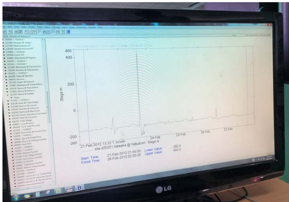
Figure 27. Tideda software user interface. (poor quality of the observations may be seen as a spike in the left side of the curve).
