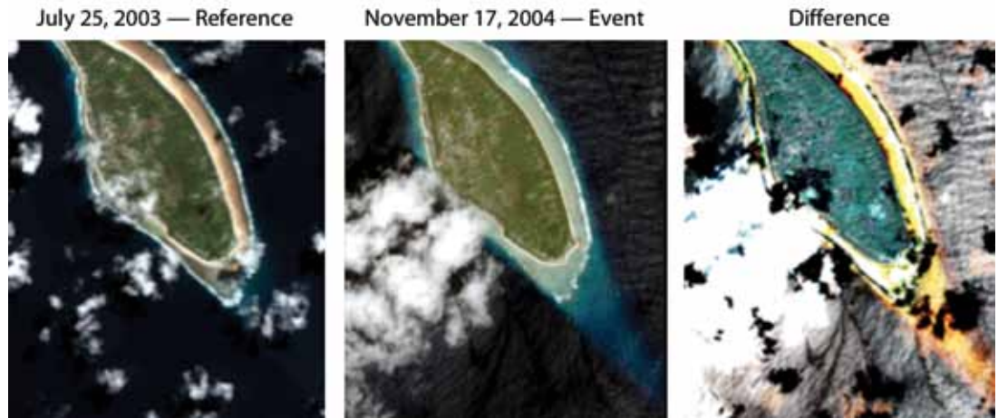
Figure 6. Image differencing, or spectral brightening, of Nikunau Island, Kiribati. The difference image (far right) shows a gold color where presumably bleaching has occurred.
