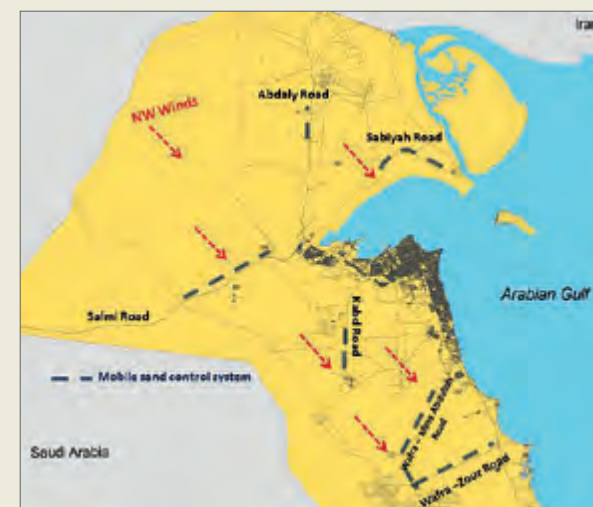
A map showing highways under threat from shifting sands: red arrows indicate prevailing winds, dotted lines indicate proposed mobile sand control systems
