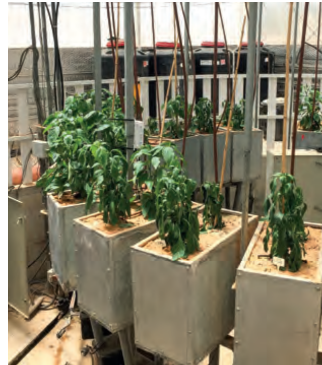
Lysimeters measure the response of pepper plants to salinity at the Wyler Department of Dryland Agriculture, Ben Gurion University
