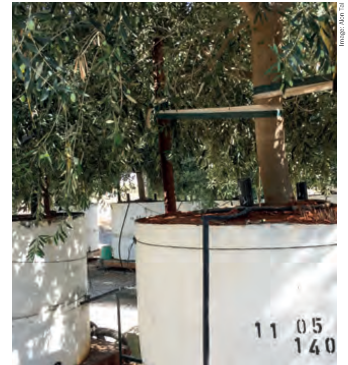
Lysimeters measure the response of olive trees to different irrigation regimes at the Ministry of Agriculture's Gilat research station
