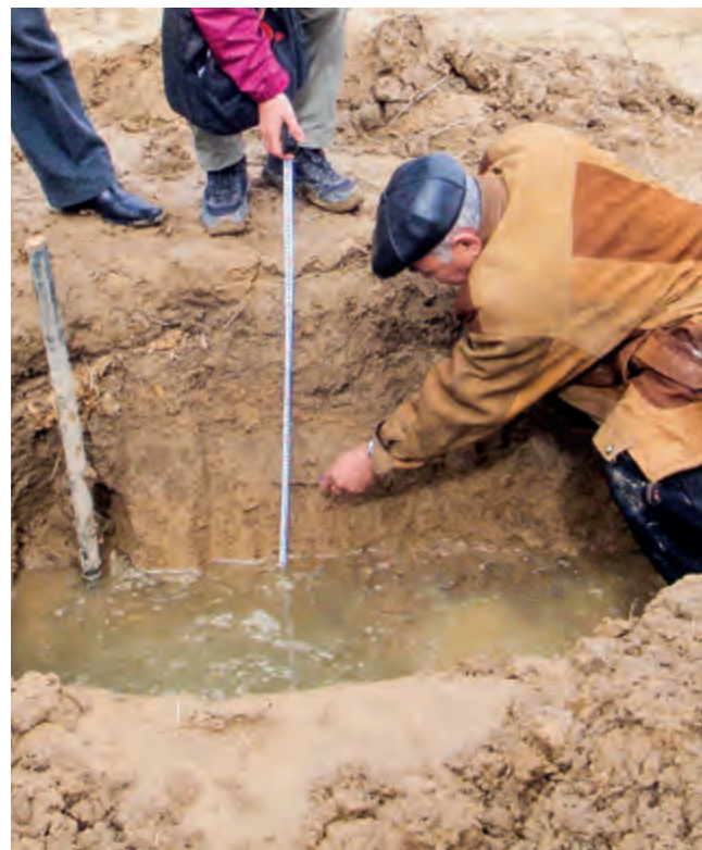
High groundwater level (70 cm from surface) was observed in Oq-oltin District, Syrdarya Province, Uzbekistan, on 21 March 2010
