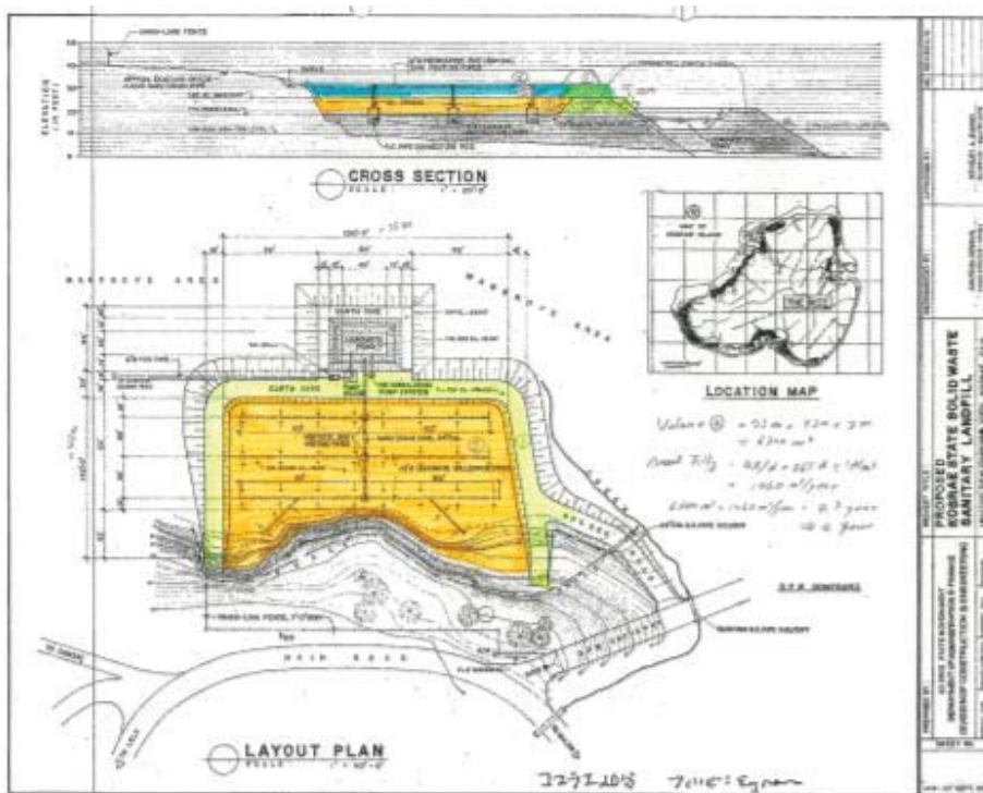
Figure 4-2 Drawings for construction of dike and access road and disposal plan for second and third phases in Toful Landfill site
