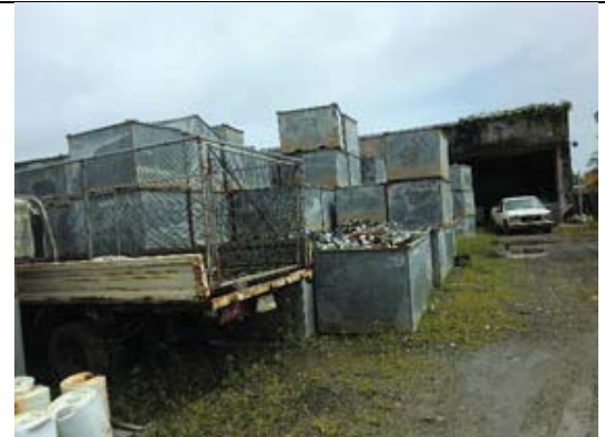
Collected glass bottles are crushed by crusher machine and crushed glass is stored on the metal containers.
