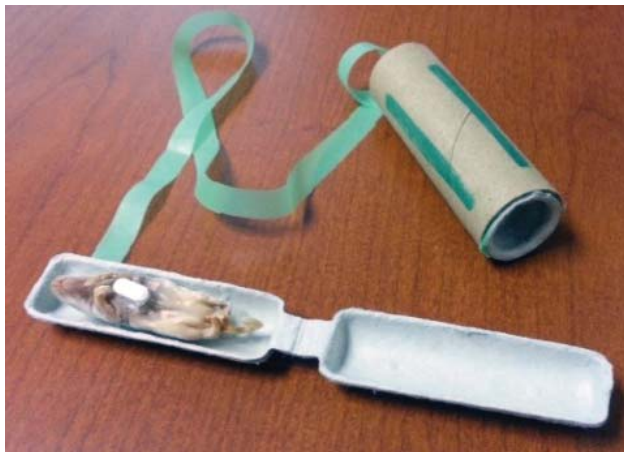
Fig. 1 When deployed, the bait capsule and outer bait cartridge tube are joined by a length of unfurled ribbon intended to entangle in the forest canopy when applied aerially.
