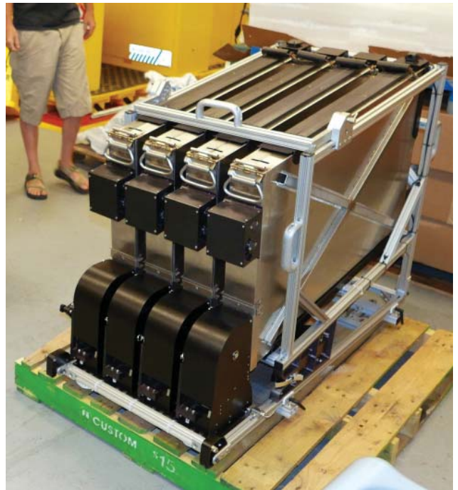
Fig. 2 The ADM is comprised of four firing units and four 900-cartridge magazines along with an onboard battery and control electronics (not visible).
