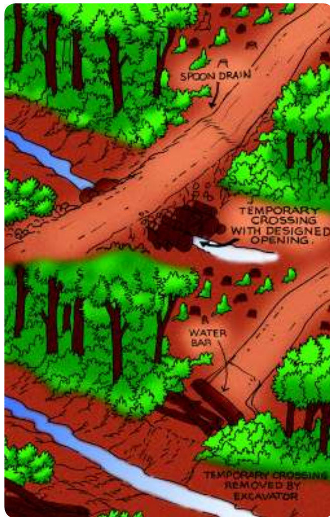
Figure 14.2: Rehabilitation of skid tracks
