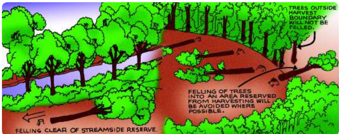
Figure 11.1: Directional felling away from buffers and retained trees
