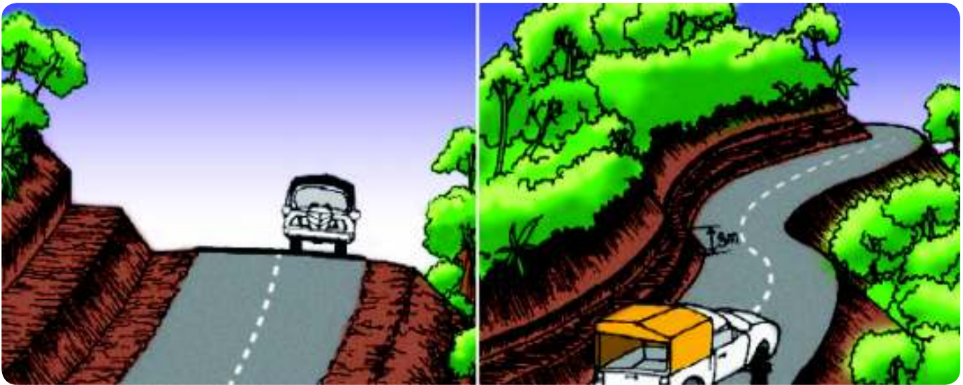
Figure 10.4: Construction of benches to improve sight distance and the stability of road batters.
