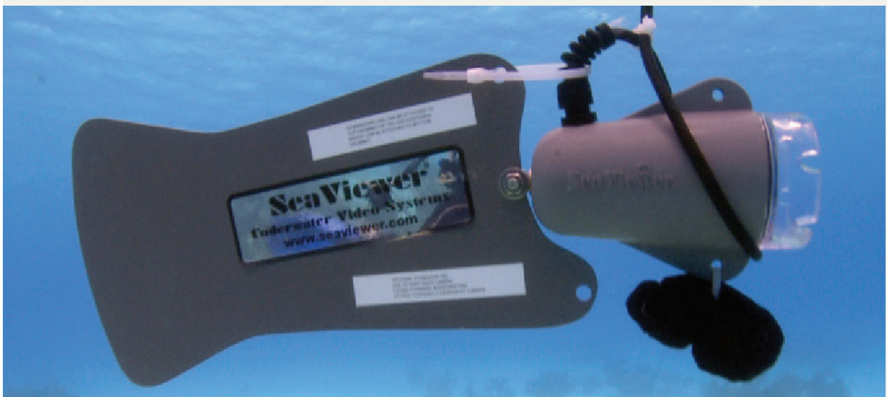
Figure 5 SEAVIEWER UNDERWATER VIDEO SYSTEM, OR DROP-CAM, USED TO RECORD BENTHIC COMPOSITION AROUND EACH ISLAND.
