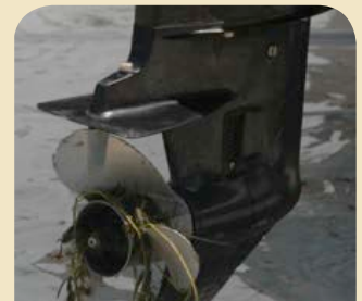
Propeller clogged with an invasive weed.
