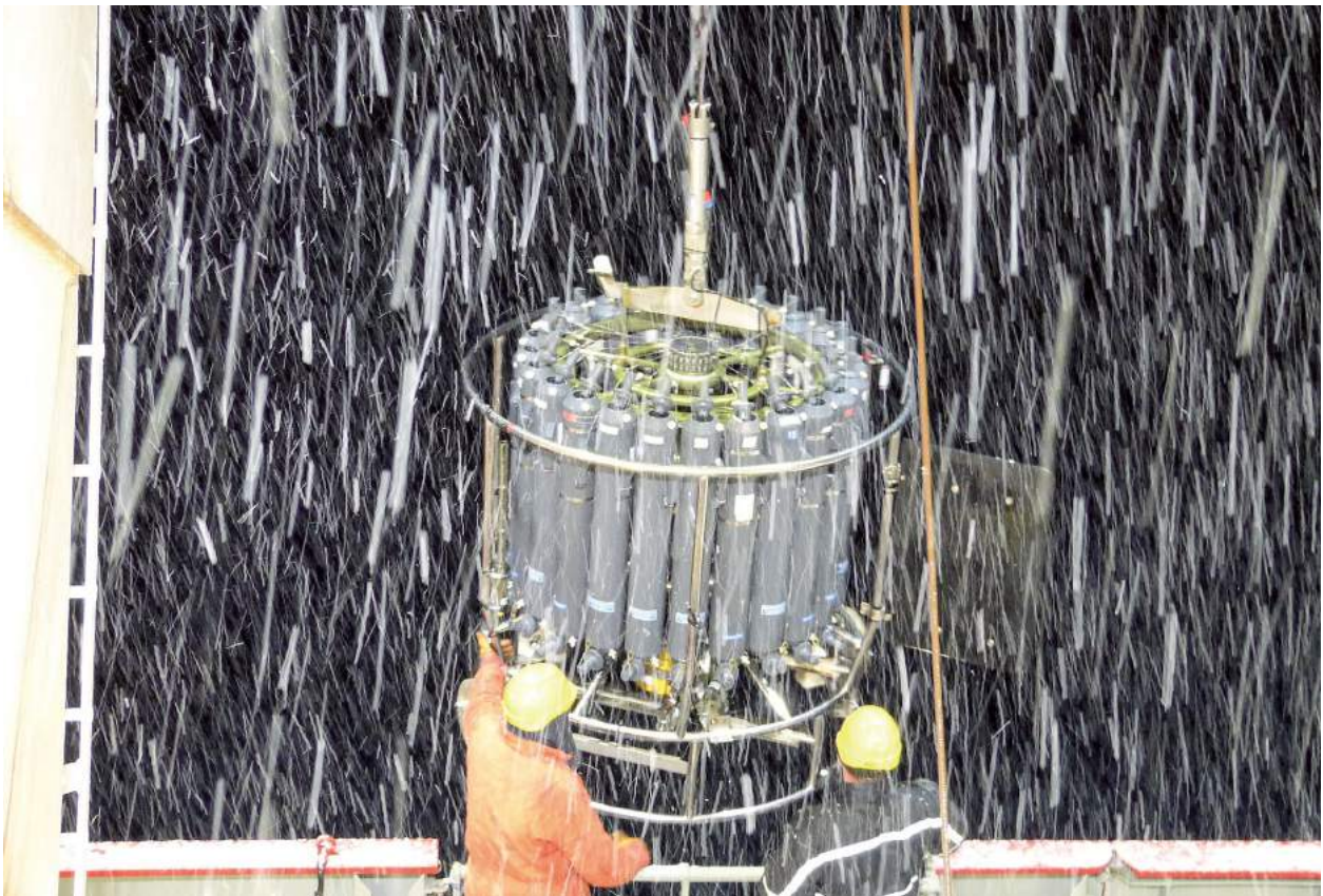
Figure 3.17.4 Scientists measuring the temperature of the Southern Ocean and collecting water samples from different depths close to South Georgia, during a blizzard. © Mike Meredith, British Antarctic Survey.
