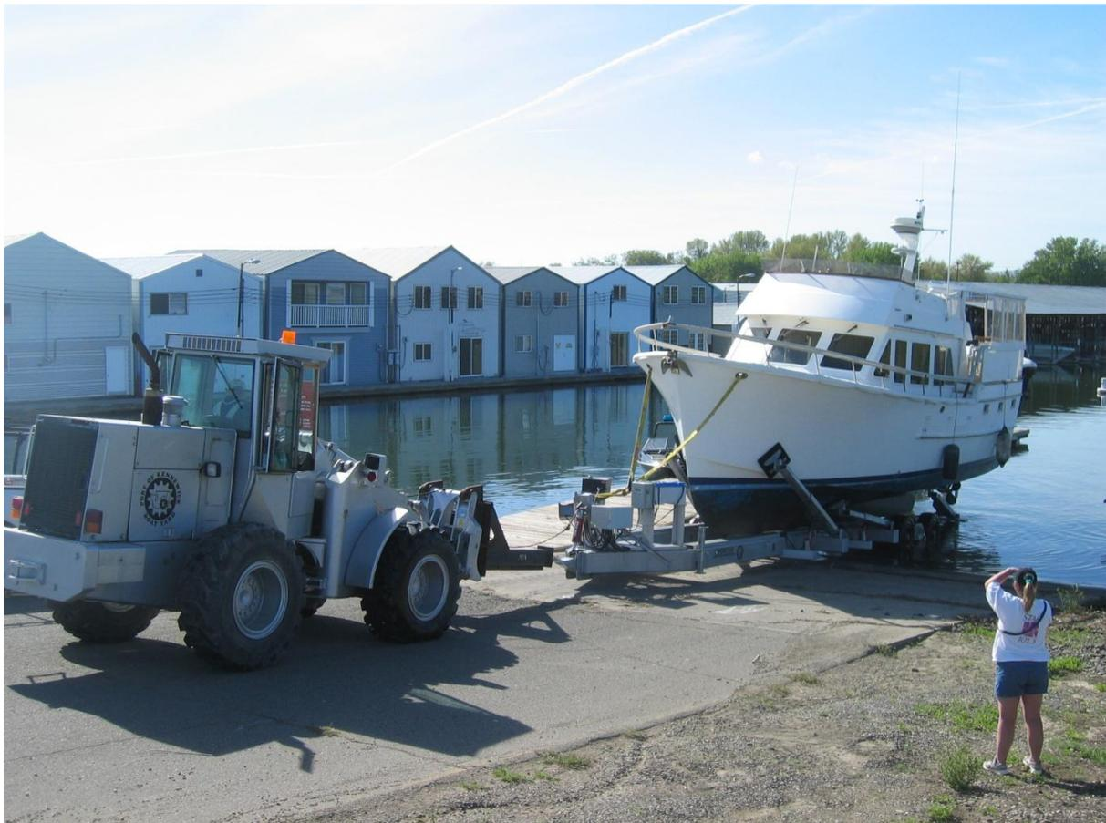
**Figure 12: Marinised hydraulic boat trailer and haulage unit to be purchased for proposed project**
