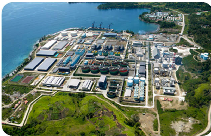
Aerial image of Basamuk Refinery in Papua New Guinea – High Pressure Acid Leaching Plant for land-based nickel laterites
