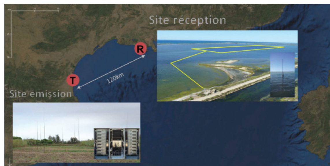
Figure 75: Example of a Stradivarius HFSWR bistatic radar (© Diginext).
