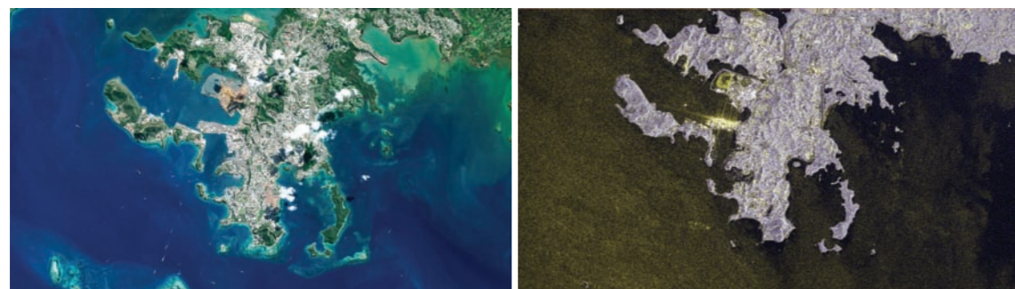
Figure 54: Left, imagery generated by an imaging radiometer; right, imagery generated by synthetic aperture radar (© ESA 2017).
