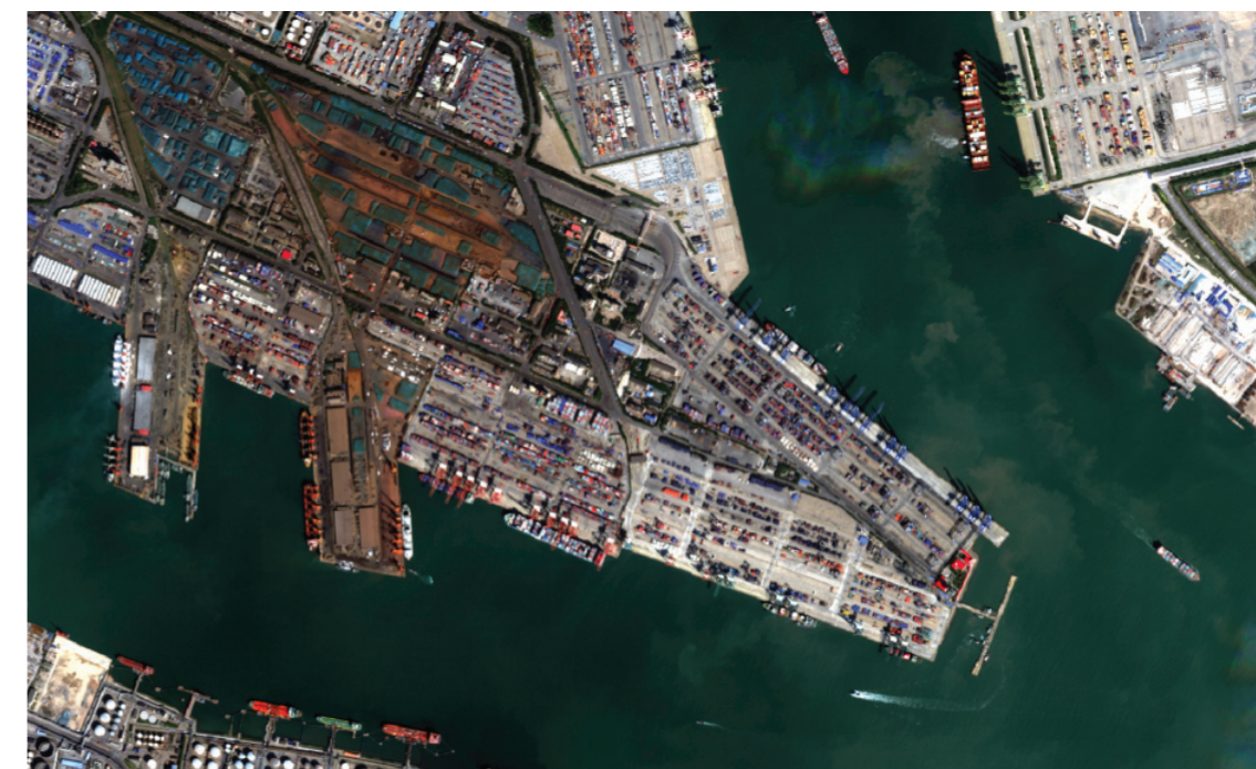
Figure 70: Example of a processed SkySat image (Calibration, orthorectification and signal boost) (© Planet Labs Inc.).
