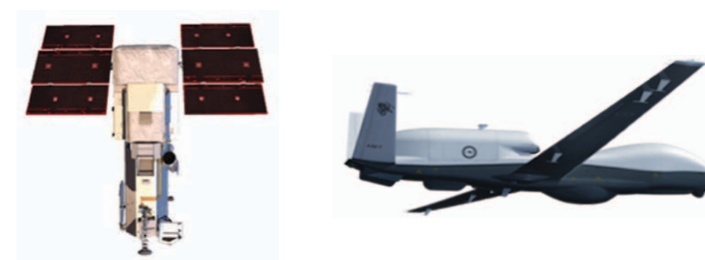
Figure 42: Left, a satellite (vector) with an on-board imaging radiometer (sensor) (source: DigitalGlobe); right, high altitude drone (vector) carrying a camera (sensor) (source: Aces Flying High).
