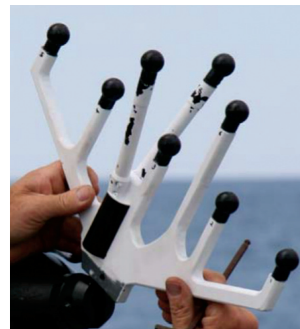
Figure 76: A hydrophone array (source: Marguer et al. 2013).
