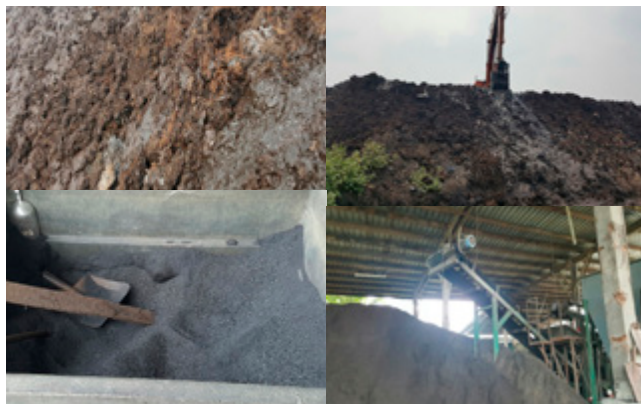
Biochar compost production using oil palm empty fruit bunch (EFB), palm oil mill effluent (POME) and biochar in the fertilizer processing factory
