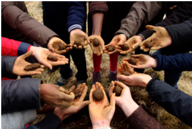
Soil texture analysed in the field by UNU-LRT trainees
