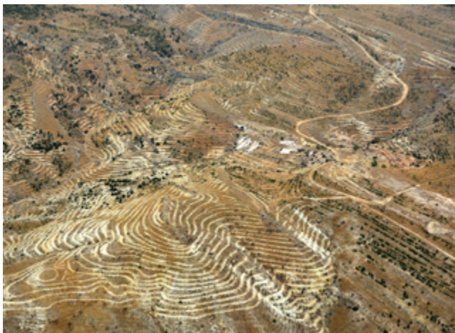
Contours for tree planting in a dry region of Turkey — an example of land reclamation on a large scale
