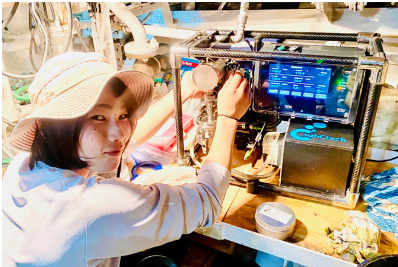
Yurie Seki changing the microplastics filters in the onboard semi-automatic sampler
