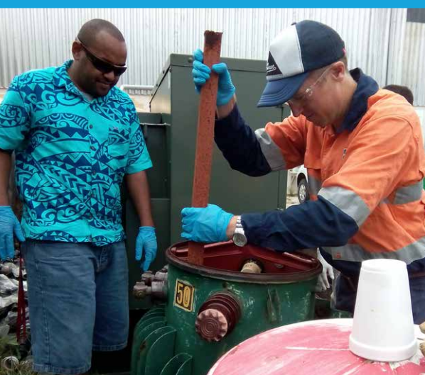
The PCB training, conducted by Mr Daniel Todd of GHD Consulting, covered best practice methods for the field testing of disused and offline transformers, online transformers, capacitors and PCB containing equipment. Photo: Jessica Zebedee/EPA
