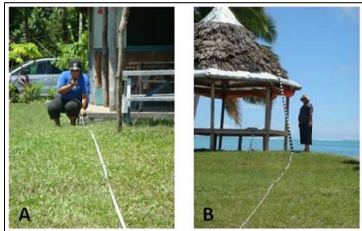
Figure D.4. A) Use the compass to find the appropriate bearing from the reference (start) point (here, the southwestern corner of the fale foundation). B) Lay the measuring tape along the transect line.
