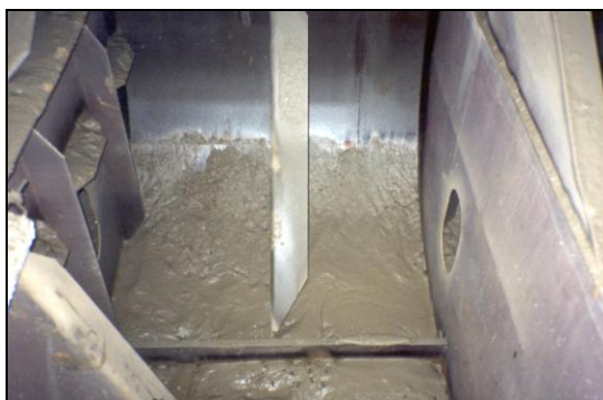
Figure A5-8: Sediments accumulated in a ship's ballast tank (Source: D Oemcke).
