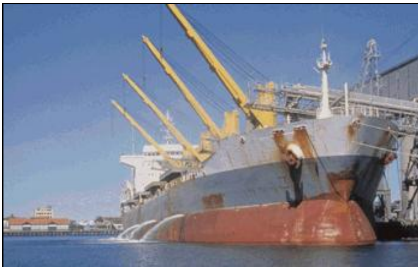
Figure A5-6 Routine ballast water discharges from bulk carrier in port (Source: CSIRO Australia)
