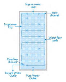
Figure 9. Solar water purifier process (Sunsure Water 2012).
