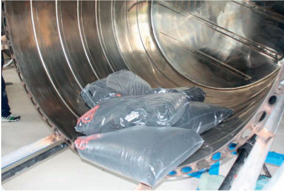
Figure 16. Mould and raw material (HDPE) in original packaging. (Photo: Niue PACC Project.)
