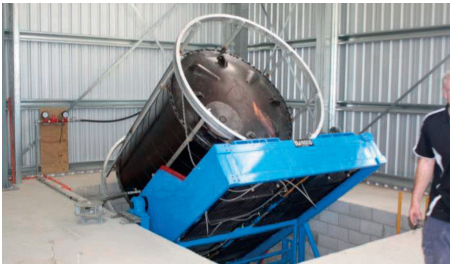
Figure 17. Moulding in process. (Photo: Niue PACC Project.)
