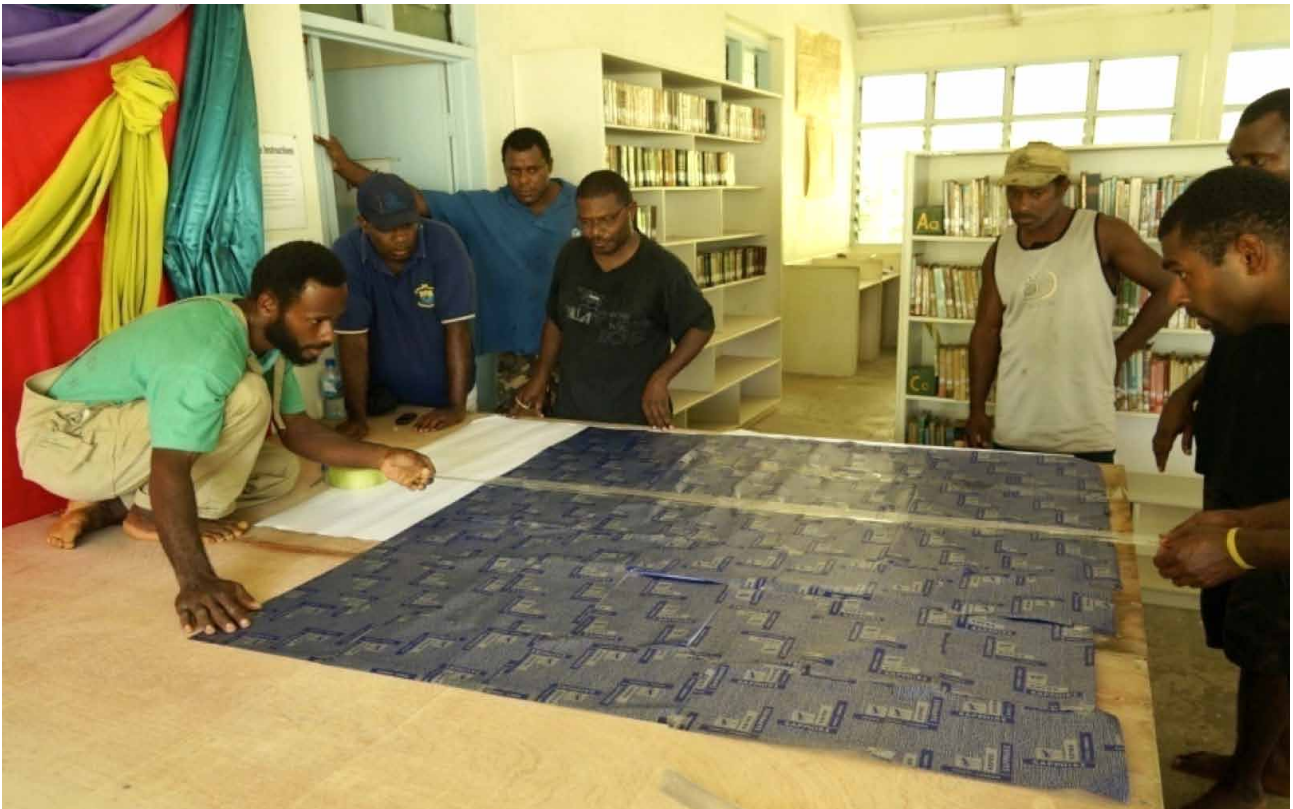
Figure 5. The carbon paper is taped onto the plywood base, ready for tracing the contour lines.
