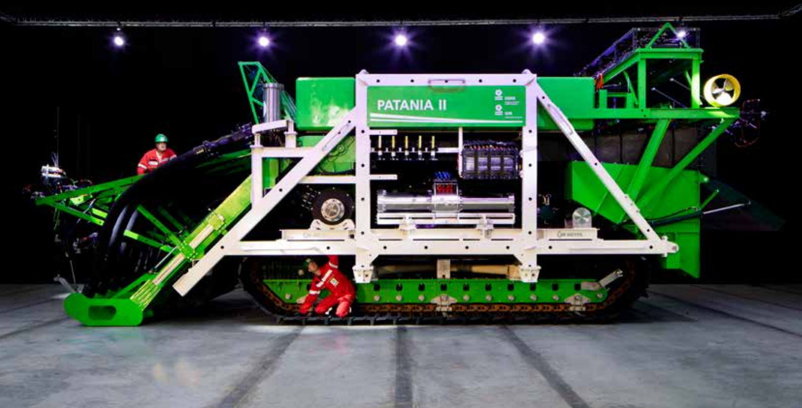
Figure 4 The Patania II which GSR is testing to collect nodules from the seabed in the CCZ Image: DEME Group: https://www2.deme-group.com/
