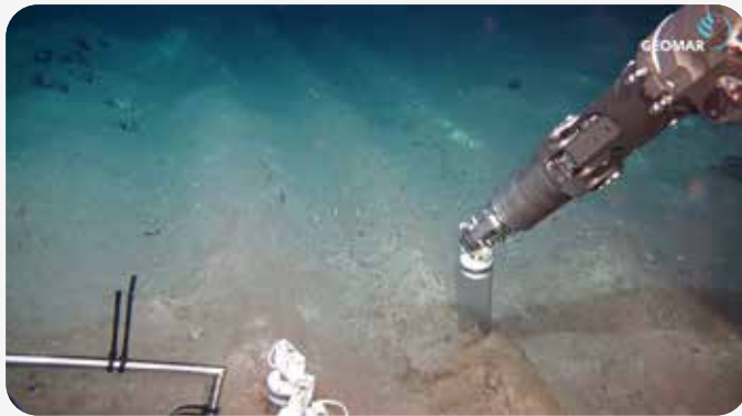
FIGURE 5: a 26-year-old test-mining track illustrates how slowly abyssal ecosystems of the deep seabed recover from physical disturbance. Image: sampling the DISCOL plow tracks. Image: Geomar, ROV Kiel 6000
