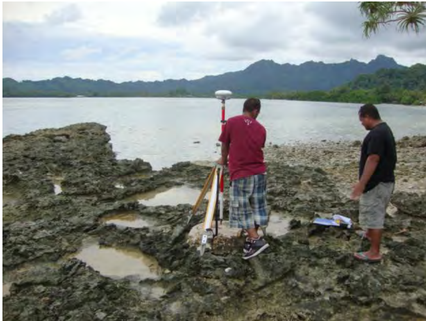
Figure 2-15: GPS being set up to collect position over benchmark S1 the fundamental benchmark for the Kosrae vertical datum.
