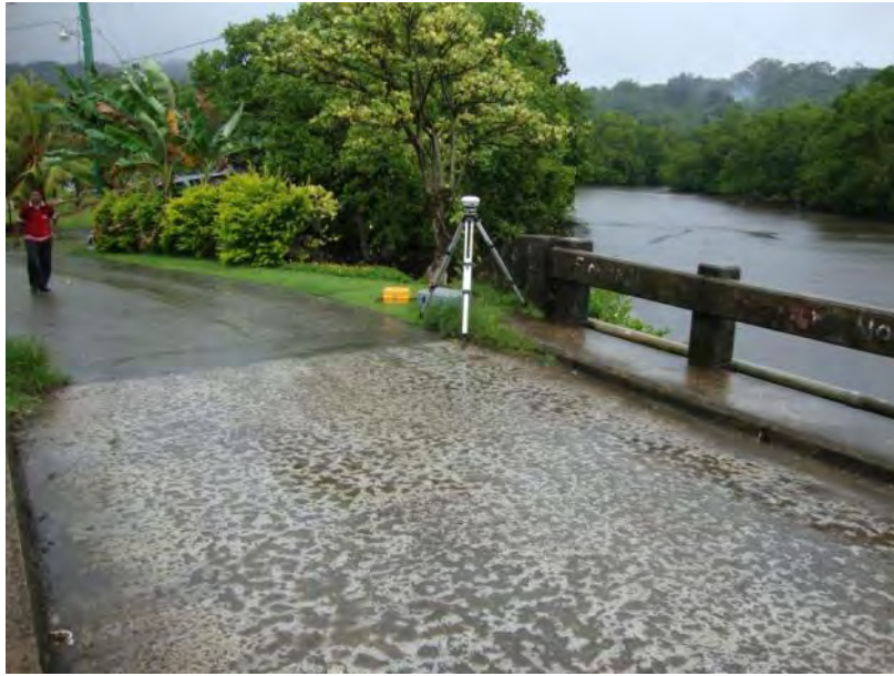
Figure 2-14: GPS collecting data over a new benchmark drilled into the concrete abutment on the NW corner of Utwe Bridge.
