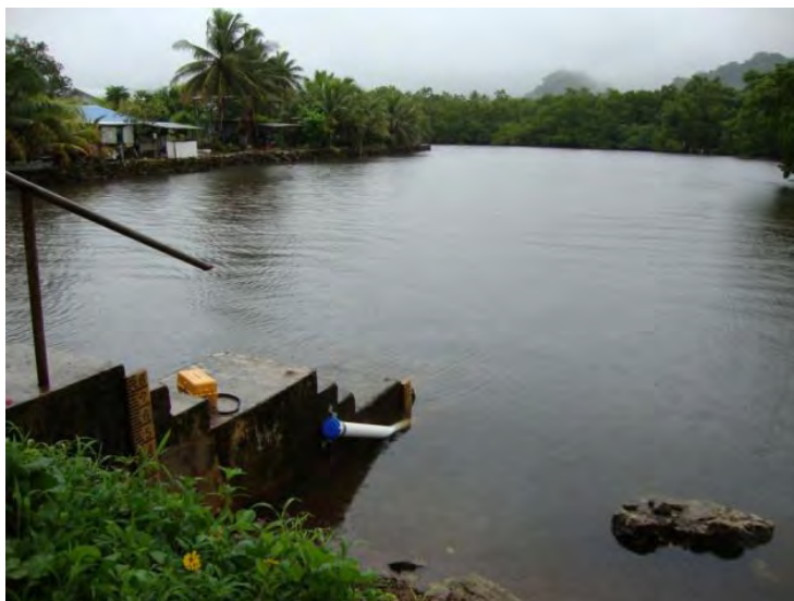
Figure 2-13: Utwe sea level station with two reference staff gauges, and PVC pipe installed.
