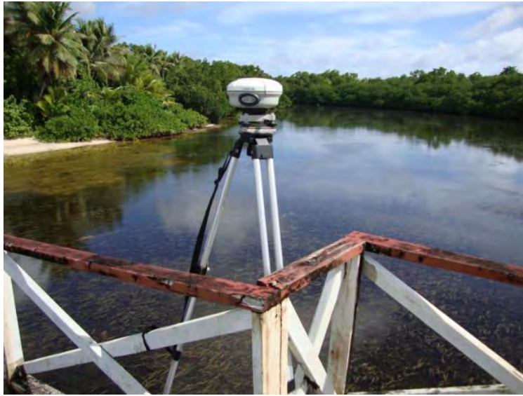
Figure 2-12: GPS collecting data over a new benchmark drilled into the concrete top of a pile on the southeastern corner of the central section of the bridge.
