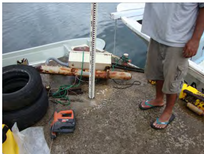
Figure 2-6: Reference benchmark on the corner of the wharf, stainless steel dynabolt in front of the staff.
