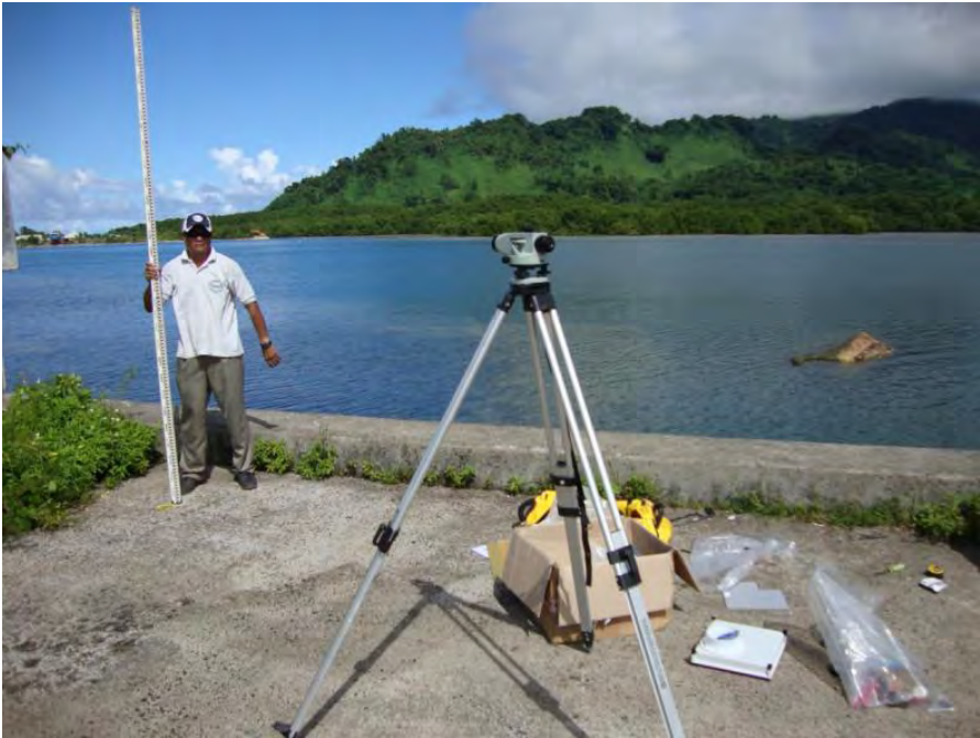
Figure 2-10: Okat Wharf benchmark, stainless dynabolt drilled into concrete deck.
