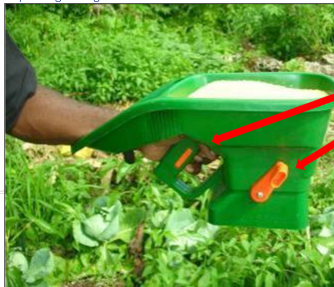
Typical hand held bait spreader showing the winding handle (a) the aperture adjustment (b) and correct grip. Set the aperture at 1.
