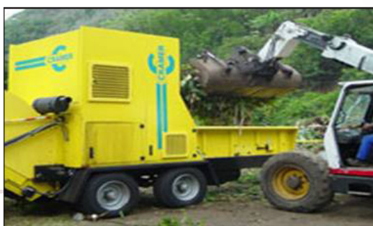
Figure 8. Technival composting facility green waste chipper. ©Technival
