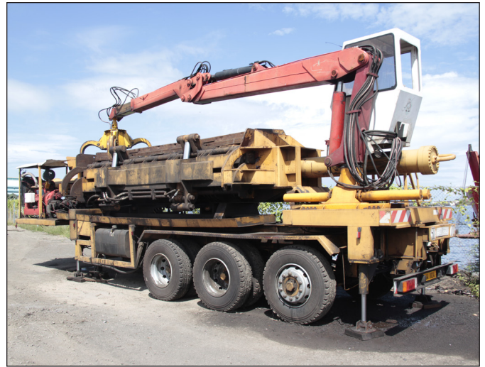
Figure 6. Mobile scrap metal compactor, CRT center.
