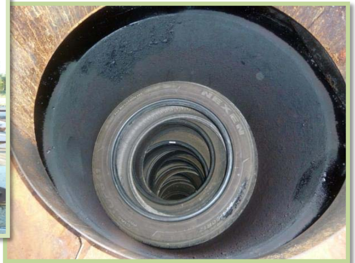
Pictured: Inner combustion chamber filled with regular EOL tyres
