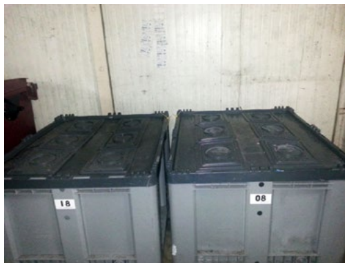
Figure 6: all waste is collected in these tubs, sealed and tagged prior to treatment
