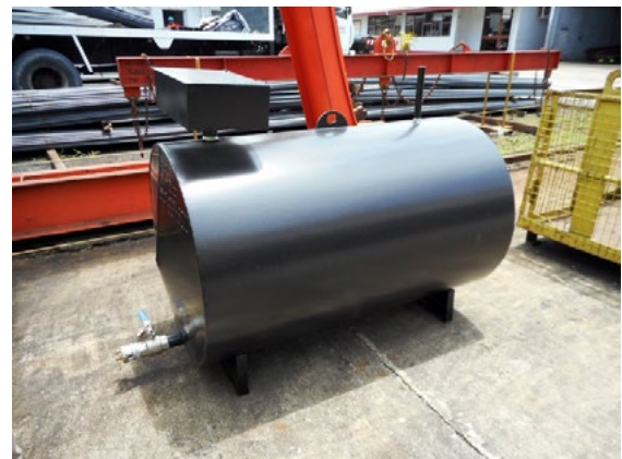
Figure 3d: Small holding tank of the type provided by Fletcher Steel to marina.
