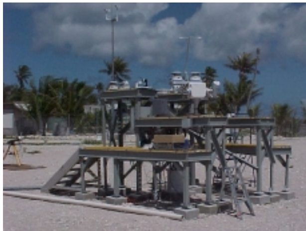
The array of instruments which measure surface radiation balance on Manus, Papua New Guinea.
