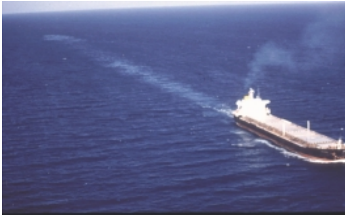
27: The discolouration left behind this vessel is from the deck washings of coal dust.
