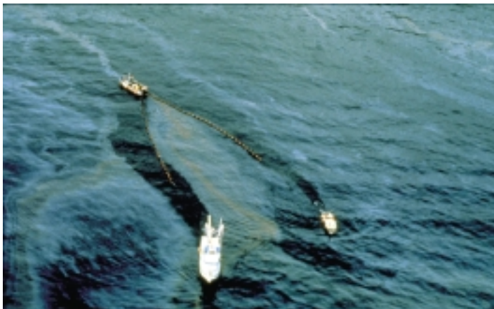
1: Boats towing a boom & skimmer through oil sheen and emulsion.
