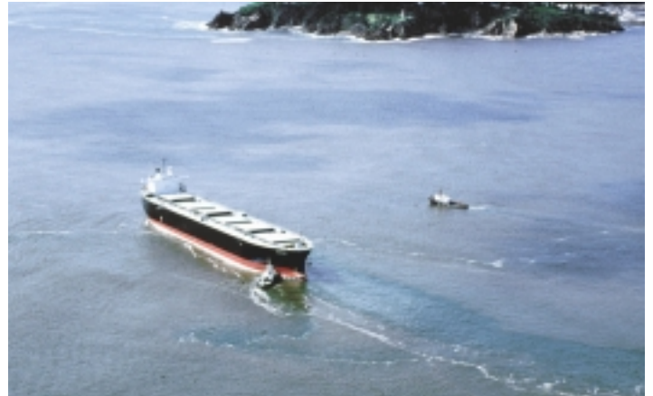
18: Vessel in shallow waters of a bay. The discolouration of the water is due to storm water run off being disturbed by propeller wash.
