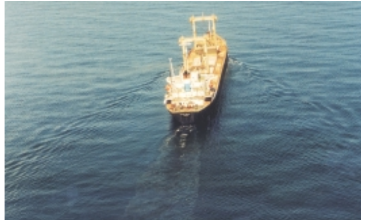
Plate 2.0: Approaching shot of vessel stern, clearly showing oil escaping from vessel.
