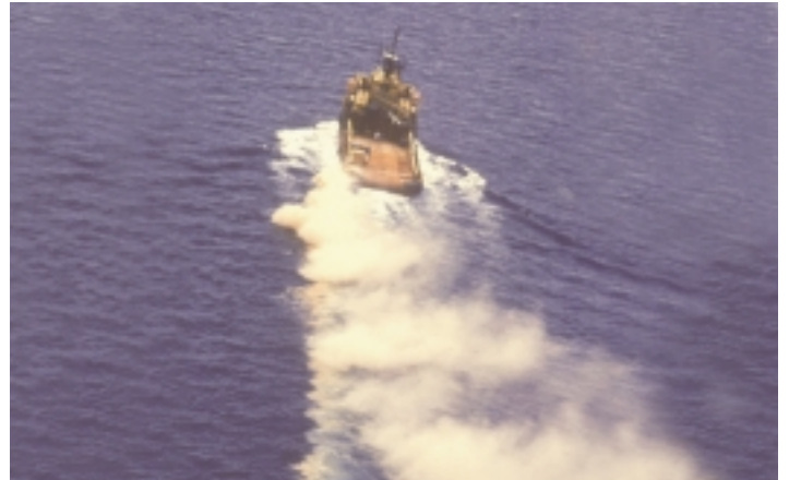
28: Vessel discharging drill mud taken from an exploration rig.
