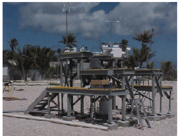
The array of instruments which measure surface radiation balance on Manus Island, Papua New Guinea
