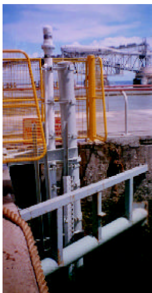
Sea Level Fine Resolution Acoustic Measuring Equipment (SEAFRAME)
