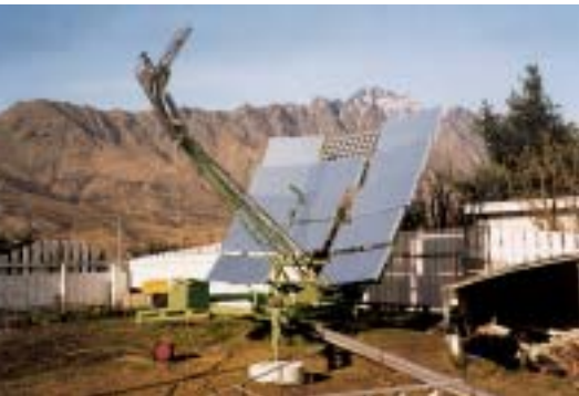
Innovative, privately developed, solar thermal collector for concentrating heat from the sun for use in home heating RS
