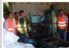
GIO Crushing machine used for baling cans as well as other materials
