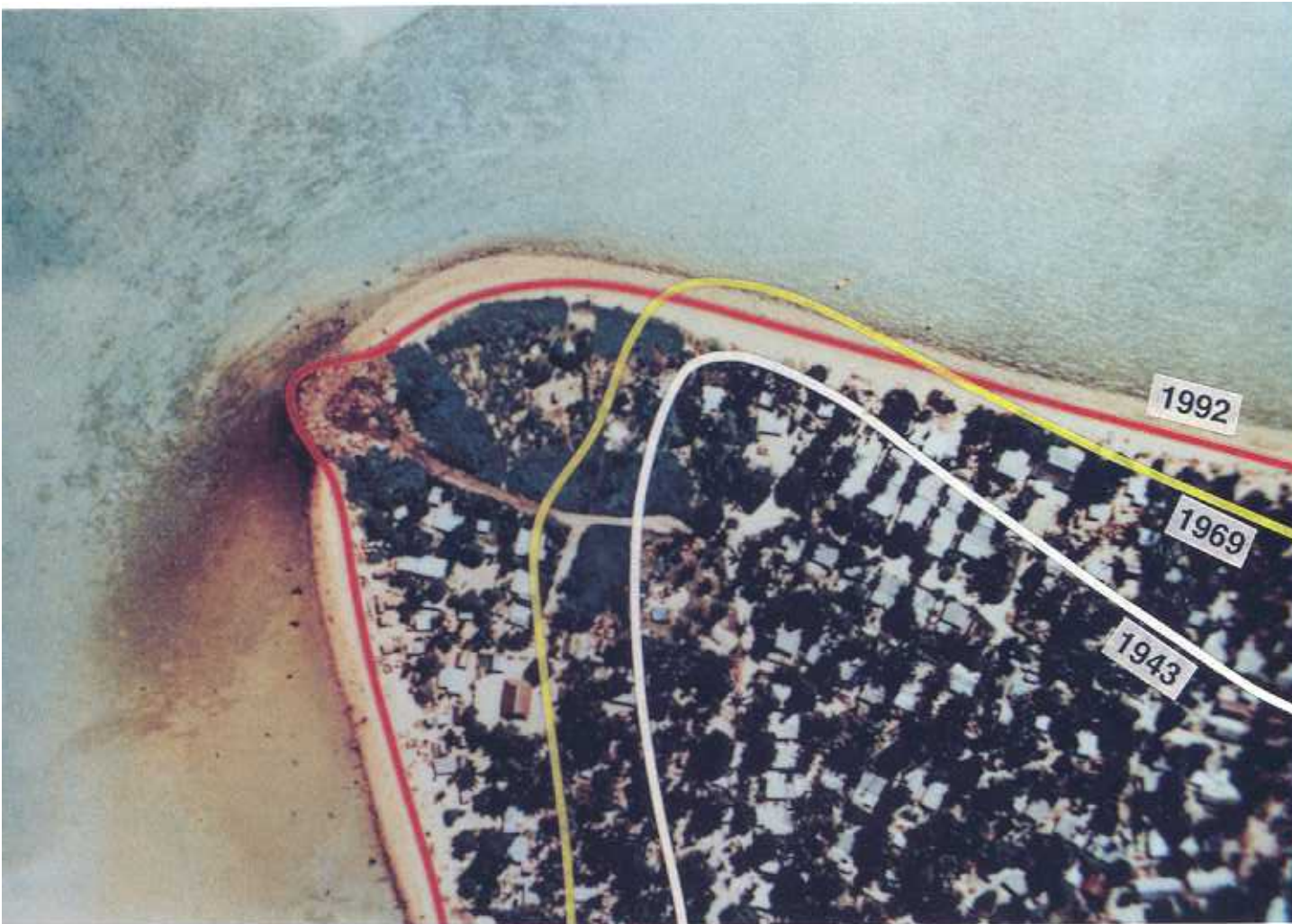
Plate 14. The positions of the 1943, 1969 and 1992 shorelines of the northwest corner, Betio islet, Kiribati, show how much the land area can change. There is now intensive development right to the shoreline, including the site being used as the rubbish dump. The coast no longer fluctuates naturally without causing an "erosion problem".
