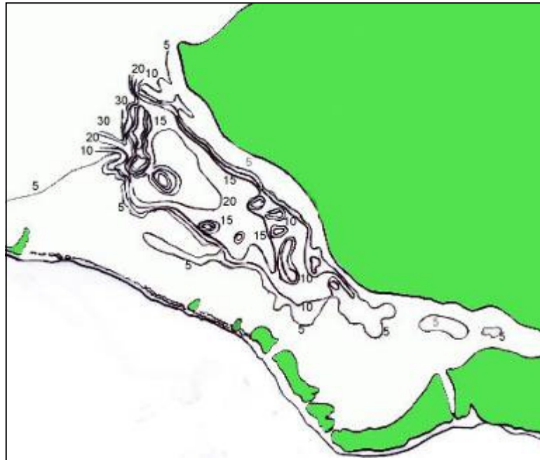
Figure 8. Approximate bathymetry of Rarumana Lagoon based on survey data and images. Contours are at 5 m intervals
