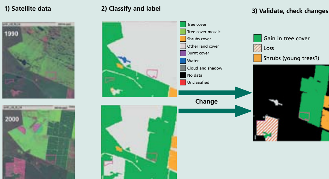
FIGURE 2.8 Example of steps used in processing Landsat data to classified land cover map and resulting land cover change, 1990–2000
