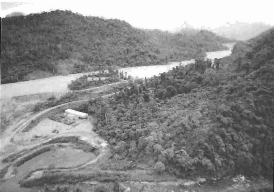
Plate 3 A river has been used for tailings discharge, and the flow completely fills the valley.
