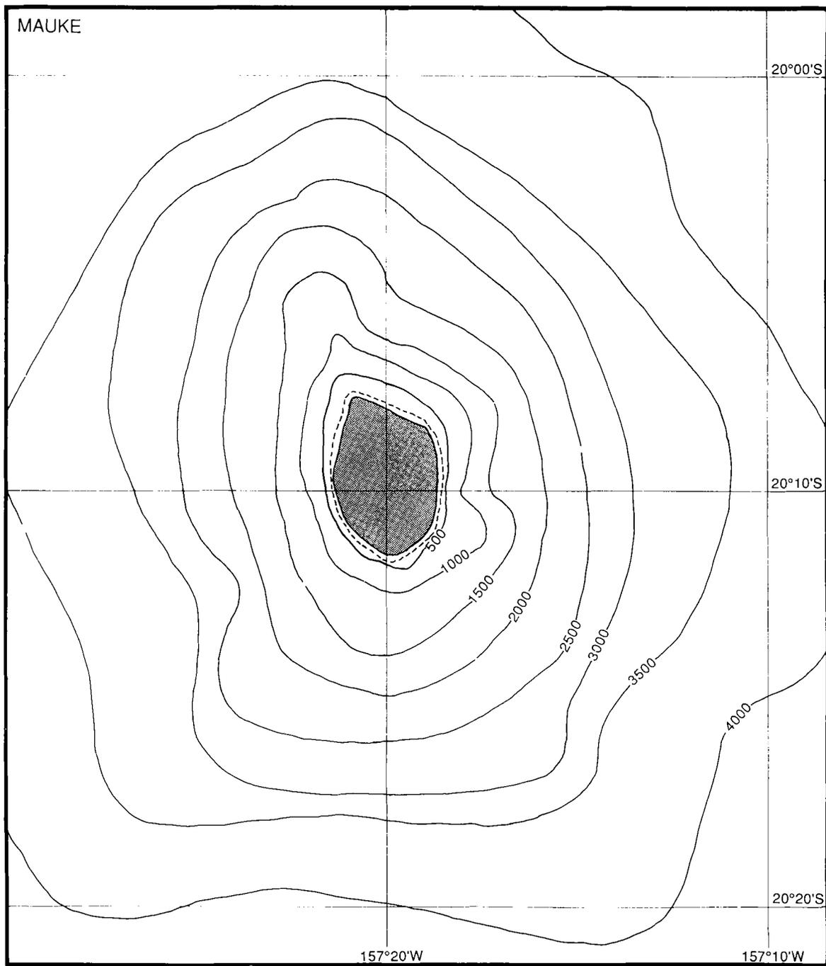
Figure 2. Bathymetry of Mauke (after Summerhayes and Kibblewhite 1969)
