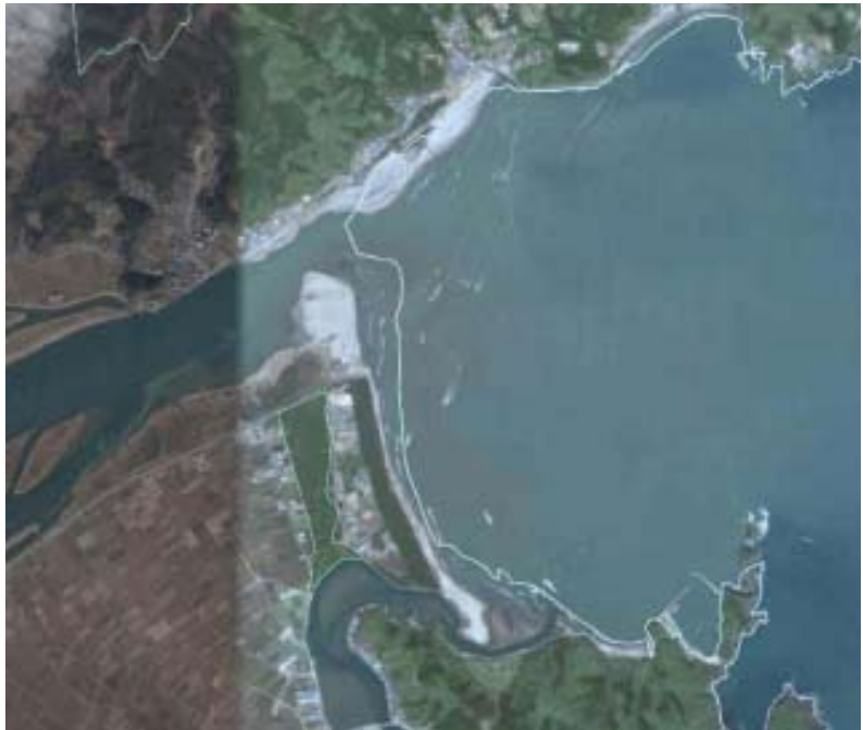
Coastal forest (center of photo) established to protect low-lying plain of Tsukihama city (Miyagi Prefecture). The town is especially vulnerable to large tsunami created by the bay. A denser, 90 meter forest forms the first line of defence, while a less dense, mixed forest, 100-190 meters wide is found behind an intervening area limited to agricultural land and buildings.
