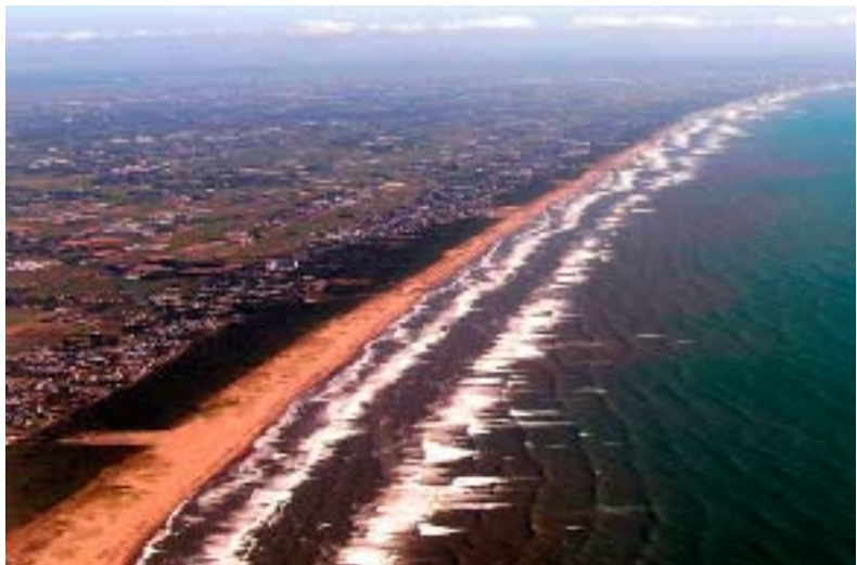
Extensive control forest in Ibaragi Prefecture on the Pacific coast of Japan. Such forests are designed to mitigate coastal hazards (strong coastal winds and blown sands, storm surge and tsunamis) and protect inland agriculture and habitation.
