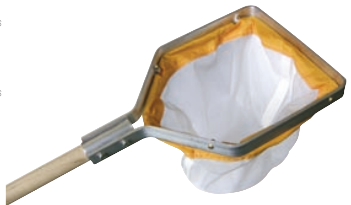
Figure 17: A hand-net for sampling small bivalves
