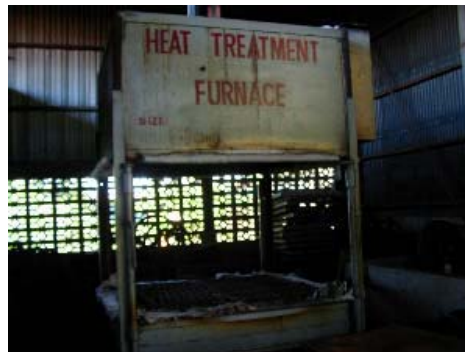
Photo 3-24 Electric oven (300 kg /cycle)
