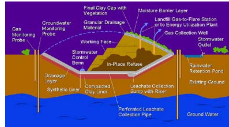
Cross section of a landfill
