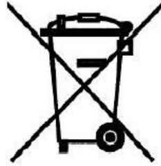
Figure III.18. Example of a sign that should appear on EEE or on their packaging.
