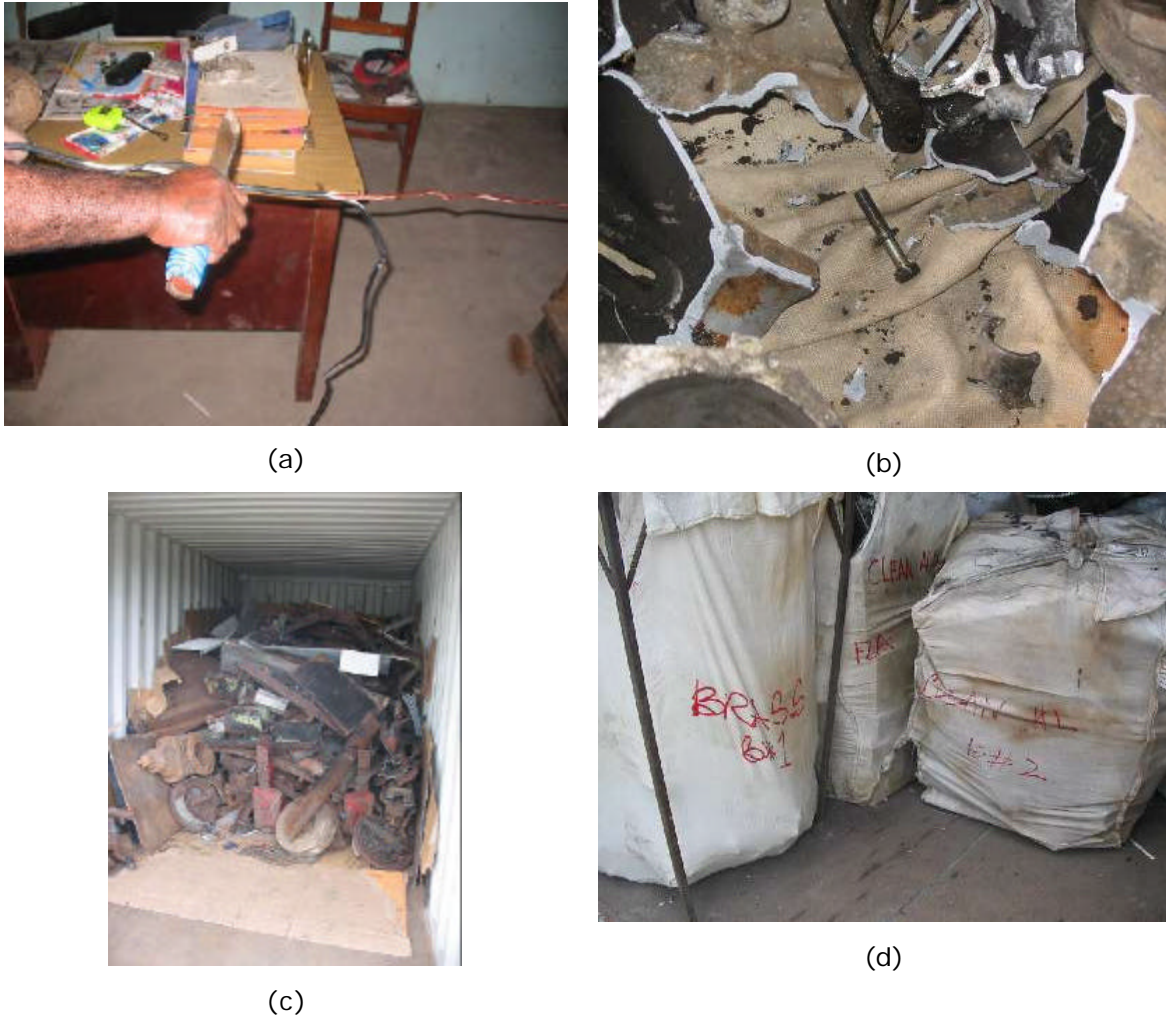
Figure II.7. Some photographs on the activity of recyclable collectors – (a) adding value to non-ferrous materials by manually extracting plastics; (b) adding value to non-ferrous metals by manually extracting ferrous metals; (c) ferrous metals ready to be exported; (d) bags of non-ferrous ready to be exported.
