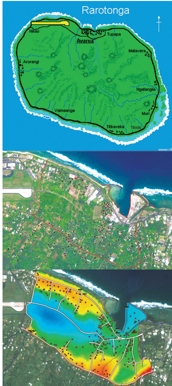
Figure VI.13: Location of the Avatiu-Ruatonga Study Area, showing (Lower Figure) Land Elevations and Locations of the 221 Structures
