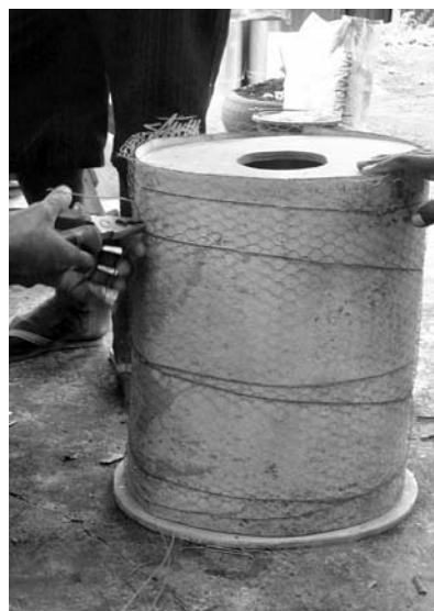
Rapemap mo fasemgud waea blong faol. Hemi shud bitim top blong flat aean long 25 mm.
