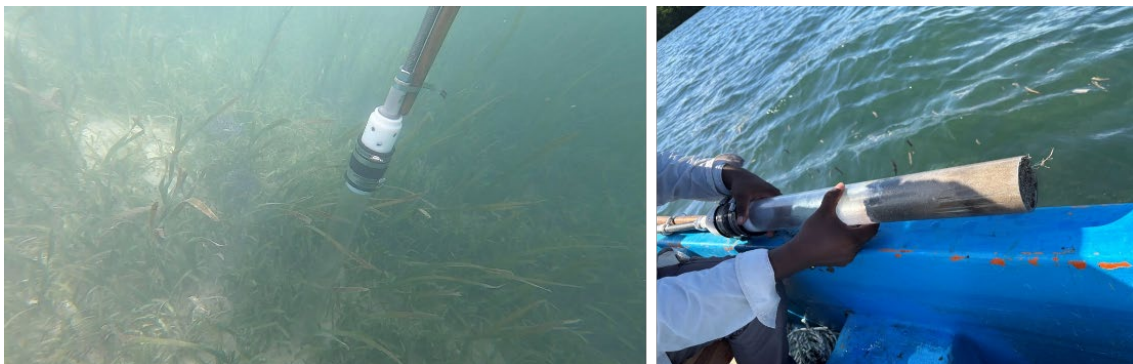
Figure 6. Demonstration of Universal Sediment Corer operation to obtain submerged soil cores.
