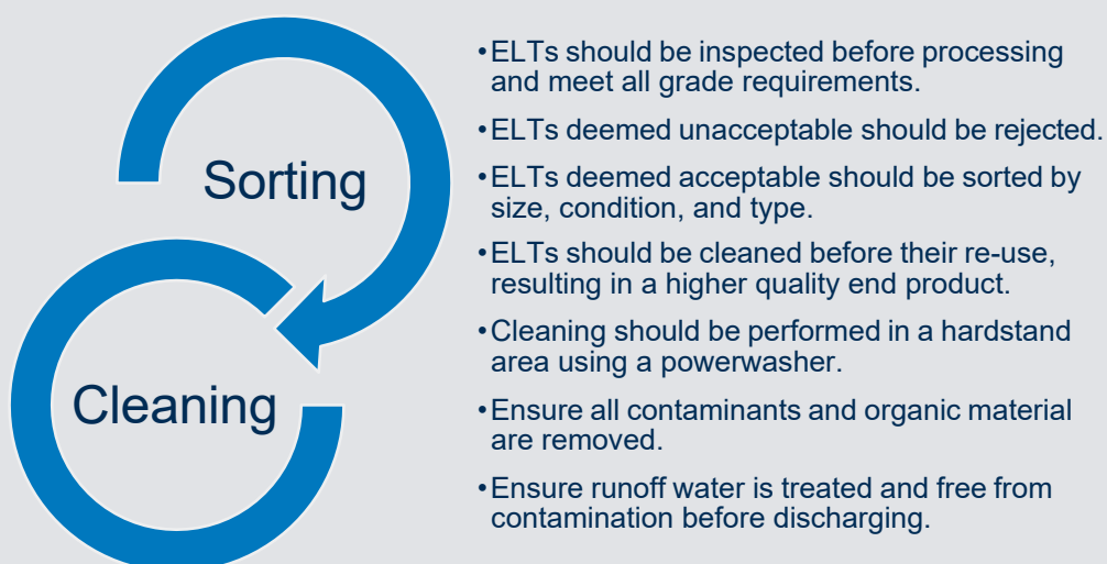
Figure 12: Pre-processing Steps for ELT granulation
