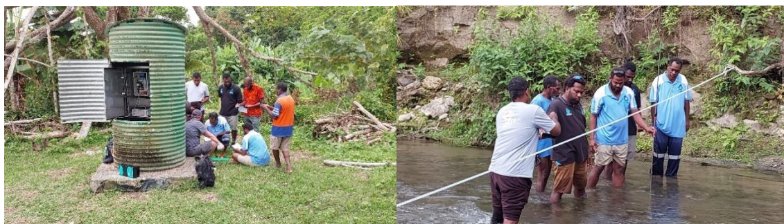
Figure A-1: Left image: Sarakata Water Level Site. Right image: Gauging exercise – small Ott current meter.
